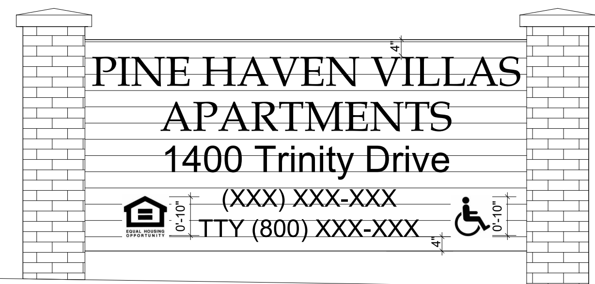
TYPICAL ELEVATION (BOTH SIDES) 1/2" = 1'-0"
